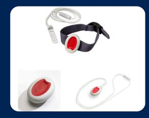
The alarm is also supplied with a wireless pendant worn around the neck or wrist allowing help to be summoned from anywhere around your house or garden (up to 50 metres from the main unit).
